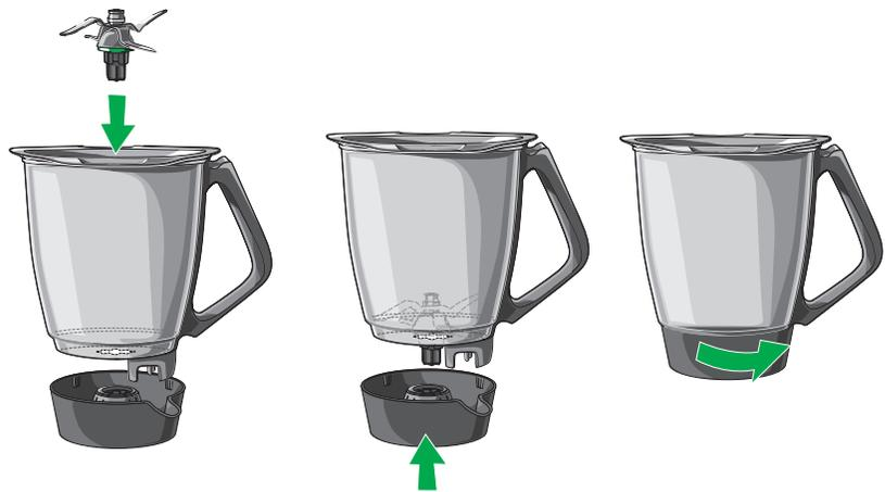
1. Ensure that the sealing ring of the mixing knife is correctly positioned under the knife bearing.
