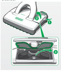
The joint connector of the SP600 is blocked.
