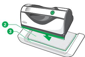
1. Lay the microfibre cloth, cleaning side down (1), onto the tray so that it is flush with the edges of the tray.
